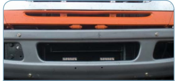
GHOST™ Multi-Mount light edge mounted to the front bumper of a large truck to offer additional white lighting.
