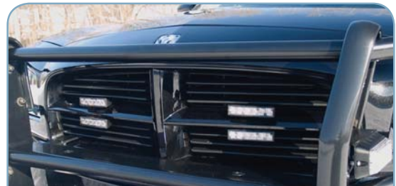
Lights can be used as supplemental Take Down lights when mounted to the grille of a police vehicle.
