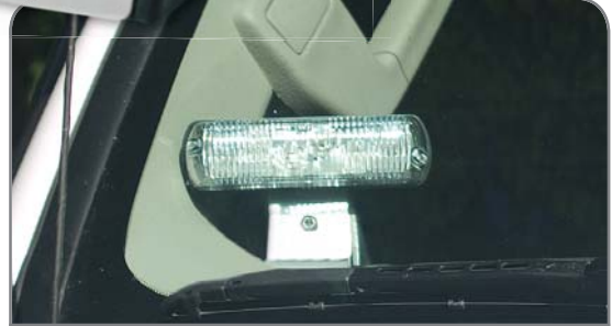
XP 63 mounted interior from window of a Ford F-250 truck provide excellent front visibility.
