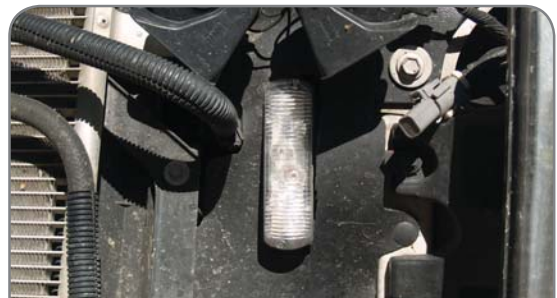
XP 63 light mounted in the grille of a Ford F-250 work truck (grille removed to show mount).
