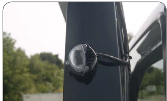
Intersector™ surface mounted on a headache rack for enhanced rear visibility & increased safety.
