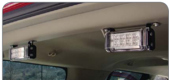
Two Predator 2™ Single Dash/Deck/Grille lights mounted to the rear headliner in an SUV.
